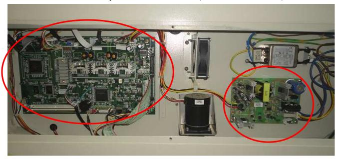
Mount AC cable (item #1) and DC cable (item #3) on power board(item #7). AC cable (Live is grey cable, Neutral is blue cable, ground is green cable). DC cable(Yellow connect to V+, Black connect to V-).
