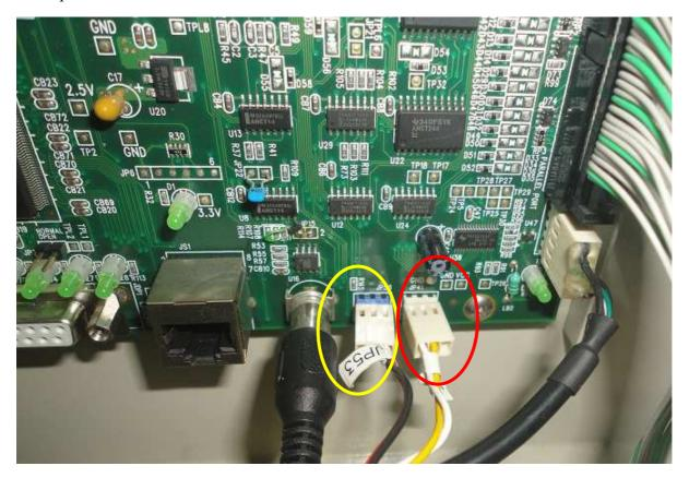
The other side of original two signal cable: JP53(yellow circle) and JP41(red circle) are on laser control pcb (the red circle and yellow circle below). Remove these two cables.
